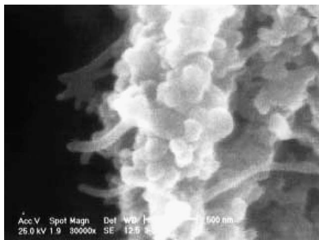
Fig. 9. SEM micrograph of the surface of the GDE modified with Nafion and PANI (GDE 2 ) recorded at 30,000× magnification.
